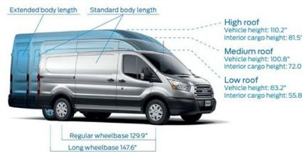
Transit is available in two wheelbases, standard and extended body lengths, three roof heights, and in chassis cab, cutaway and wagon configurations.
